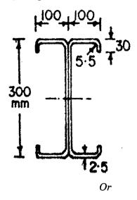
8. The beam having cross-section shown in Figure is laterally supported at 1 m interval. Compute the moment of resistance, taking  $M_1 = -0.7 M_2$ . Assume missing data.
