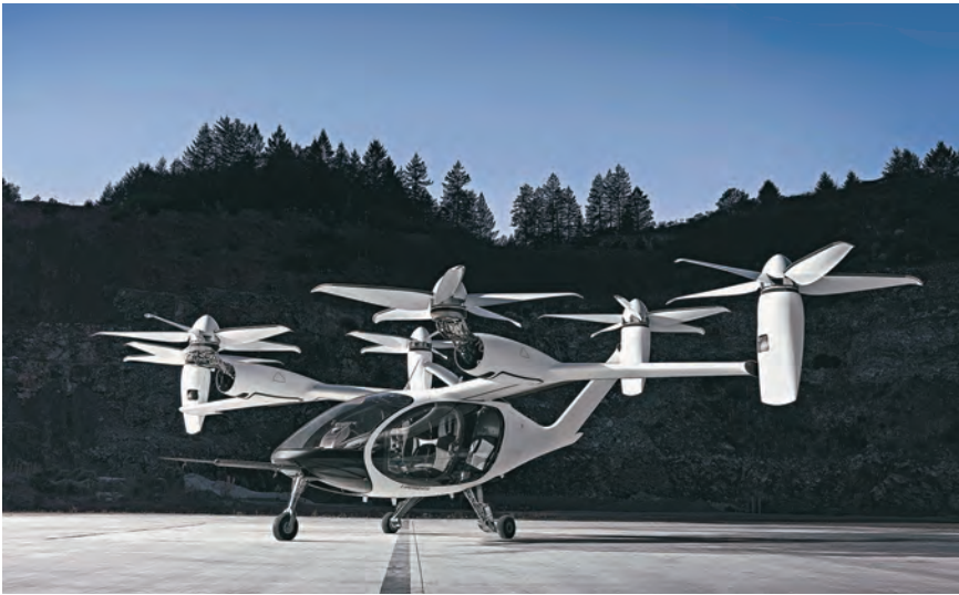
Joby’s aircraft has six propulsion units that enable it to stay aloft even if a motor fails. The propeller blades are shaped to make it quieter than a helicopter when taking off or landing vertically, and virtually silent when tilted forward in flight
